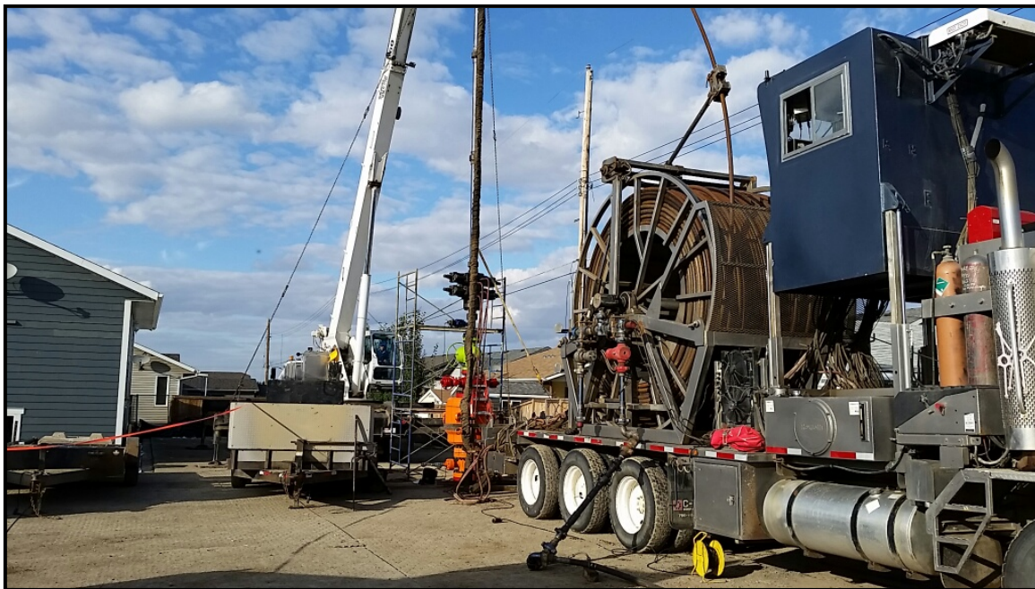
Tenwell Gas & Oil Co. Ltd. 00/09-36-050-07W4/0 2014 September 13 Coil Tubing Operations
